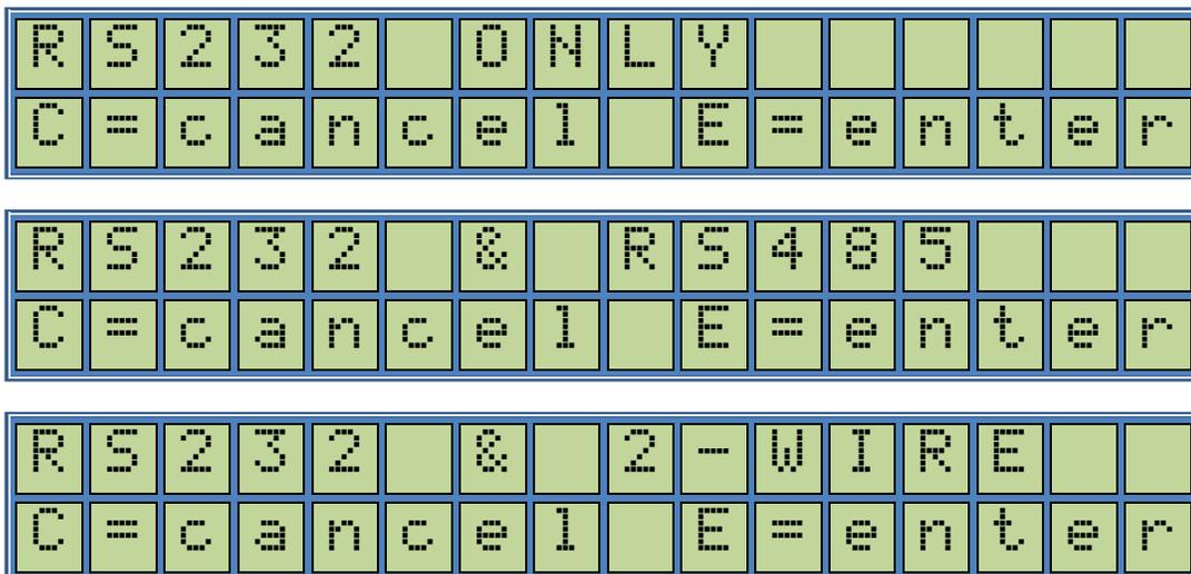
This is for setting Serial Port Type. The system can communicate in RS232, RS485 and Current Loop (Gilbarco 2-wire) standards.
