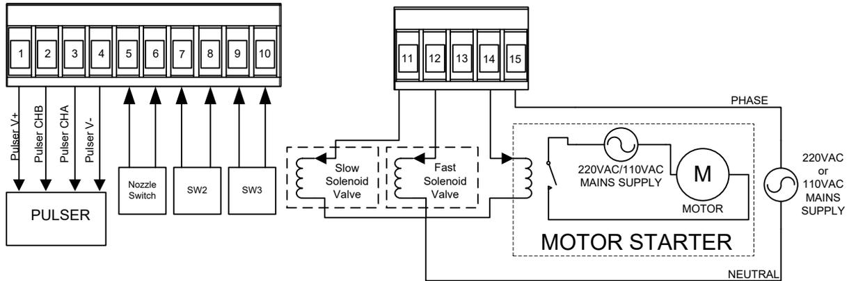
**NOTE: For multiple hoses/dispensers, the TP3-14 RED Motor Starter wires MUST NOT be combined. Use a relay such as FINDER 48.31.8.120.0060.SPA or equivalent to isolate separate dispensers**
