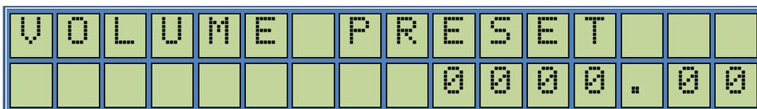
Again by using the number keys followed by the
