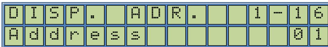
As the selection appears on the screen you can preset the figure by typing the number keys to the desired amount. The number pressed enters the screen from right and the previous number in the screen shifts to the left by one digit.
