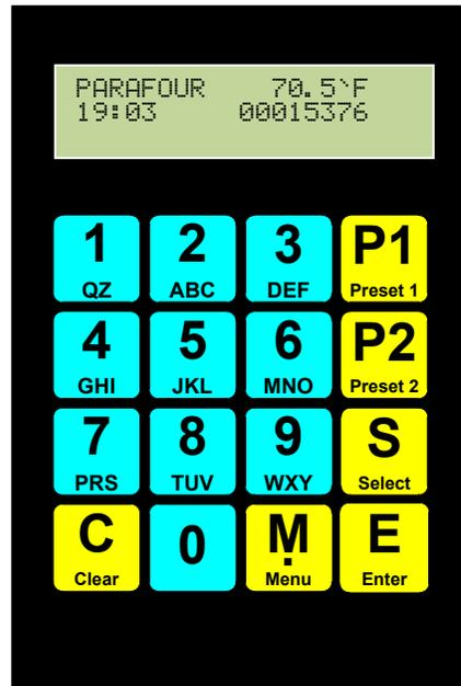
For normal operation, there is no need to activate any options with the keypad in order to dispense fuel. Simply press the "PUSH-TO-START / STOP" button to initialize dispensing, or if equipped with a "LIFT-TO-START" nozzle boot, then lift the nozzle to start. The display should first read 'INITIALIZING.....' And then change to "FUELLING..." when the display has reset and the pump has been turned on.
