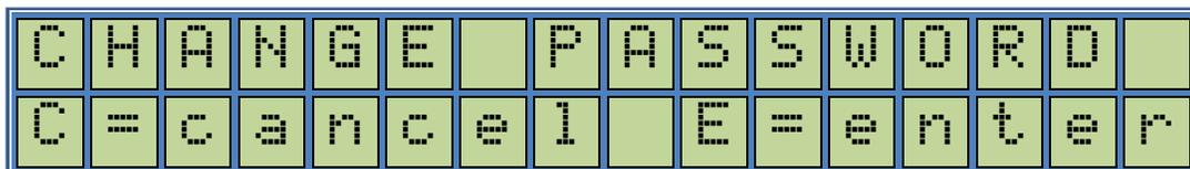
This function is for changing the technician password which is necessary for accessing to some of the system settings.
