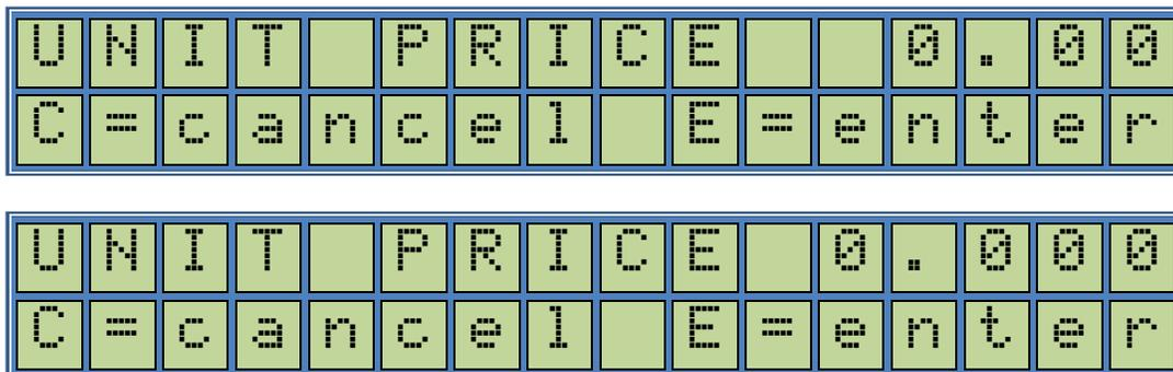
This is for setting the dot position on Volume display. Pressing the
