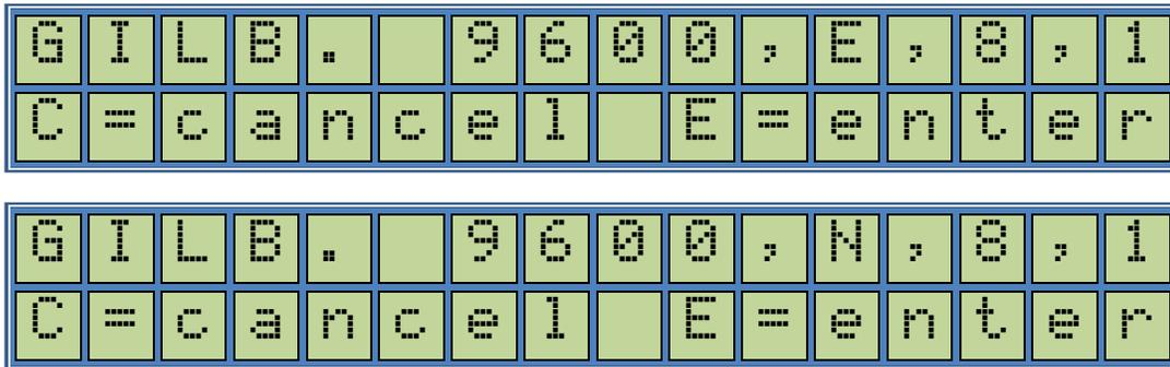
This is for setting Serial Communication Protocol Parameters. The system is capable to communicate in Gilbarco Protocol. You can use standard 5787 Gilbarco Baud rate as well as 9600 industry standard baud rate as shown above.
