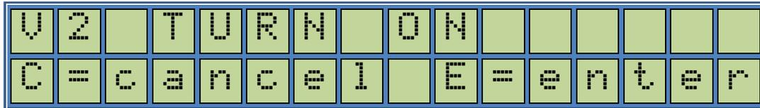
This is for setting the Amount in Volume after which the second solenoid valve (fast valve) should open during the beginning of product delivery. *This function is used ONLY with "2-SOLENOID" Preset option. For SINGLE SOLENOID OPERATION, this setting is not required.*
