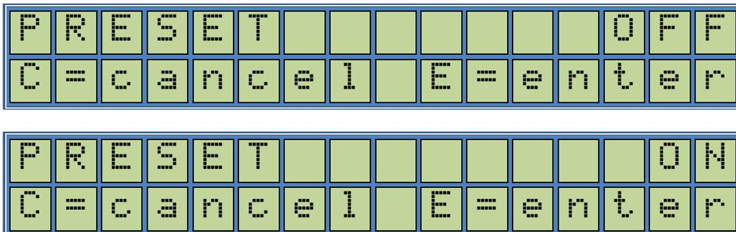
The dispensing operation can be with or without preset function enabled. When turned on, the user will have the ability to make a preset sale either based on a fixed amount or a fixed volume.
