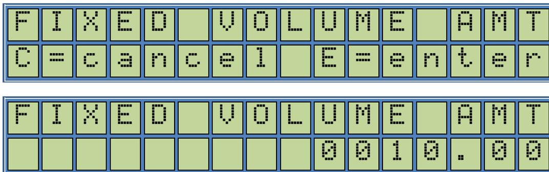
As stated, the previous setting enables or disables the Fixed Delivery Volume Function. Here we define the fixed delivery amount. Number keys will be used to set the desired amount. To finalize the fixed amount programming, you should press **E** key and the display will return a message like "STORED", which will store the new value into the non-volatile memory.
