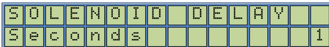
As the selection appears on the screen you can preset the figure by typing the number keys to the desired amount. The number pressed enters the screen from right and the previous number in the
