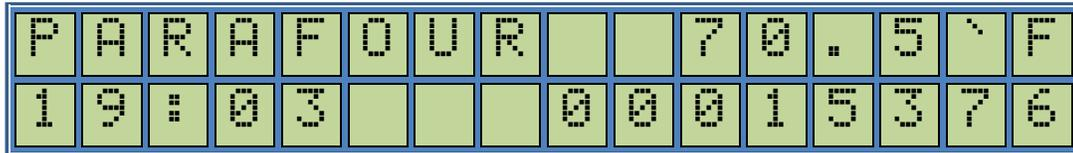
That is the company logo and the temperature at the first line and the time and the totalizer reading on the second line. This is the basic dispensing **“Operating Mode”** message. The dispenser will ONLY dispense fuel when the display shows this message. Therefore, after programming configurations, you must return to this screen mode for routine fuel dispensing. Please note the temperature will only be shown if the ATC is enabled.
