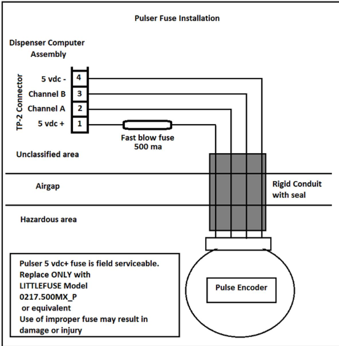
**WARNING:** The pulser, conduit and cable are a not a field serviceable factory assembly.
