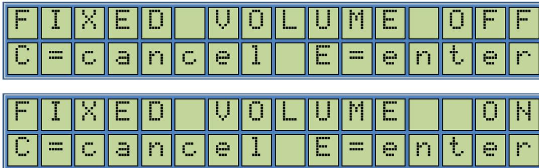
This function serves usually for calibrating and adjustment cycles. The dispenser can be set to dispense a fixed amount of volume at each delivery without using the preset function and its capabilities. If this setting is turned on, each delivery made will be based on the quantity set at Fixed Volume Amount Setting (next menu item). Pressing the **S** key will cause the screen to switch between the above indicated conditions.
