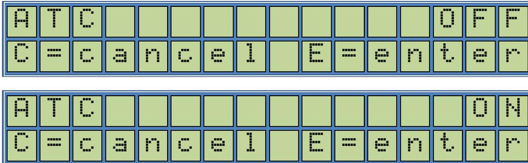
This is for enabling or disabling the ATC operation. Pressing the
