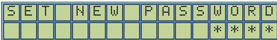
Enter the new user password by using the number keys. The user password is a 4-digit number and it should be followed by **E** key to be stored into the nonvolatile memory.
