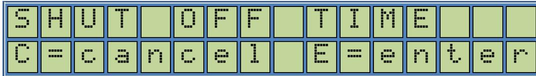
This is for setting the Shut off time i.e., the allowed time for the motor and solenoid valve to keep open during a product delivery as if there is not any product flow.
