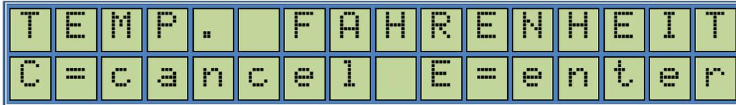
This is for setting Temperature Display readout type. Please note that if ATC is not enabled there will be no Temperature Readout on the main display.
