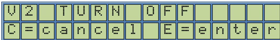
This is for setting the Amount in Volume before which the second solenoid valve (fast valve) should close during the termination of product delivery. *This function is used ONLY with "2-SOLENOID" Preset option. For SINGLE SOLENOID OPERATION, this setting is not required.*
