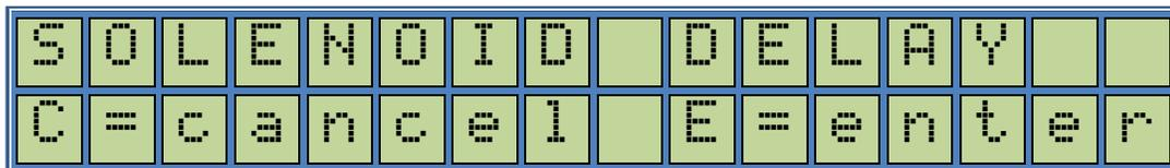
This is for setting the Solenoid delay time i.e., the time in seconds between the motor start and solenoid valve turning on at the beginning of the product delivery. *The recommend setting is for 2 seconds longer than the pump motor starter delay.*
