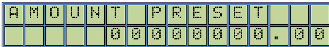
By using preset buttons the value pre-assigned will be added to the value on the screen and displayed both in the keyboard screen and sales field of the main display where, the volume part is automatically blanked out for better visibility. To change the preset from amount to volume or vice versa, the user should press both buttons at the same time. This will result in the following screen;
