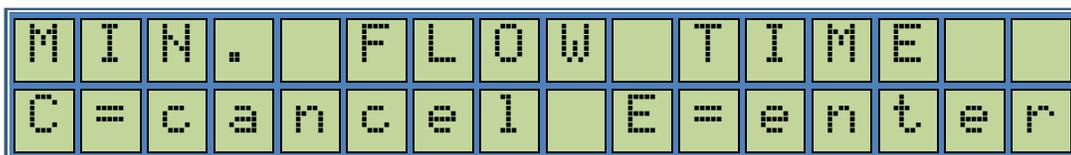
The minimum Flow Rate Time is the allowable limit in second for the dispenser to continue normal operation when the flow rate falls below the minimum flow rate set. This option is only valid if the minimum flow rate control option is enabled.
