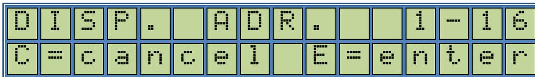
This is for setting the Dispenser Address. This is important if the dispenser is included into a communication chain. Default Dispenser Address is 01.
