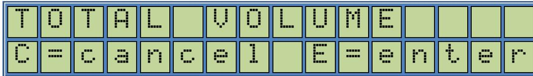
This is for reading the total Volume dispensed by the dispenser since initial setup. The volume indicated here should correspond to the volume indicated when the dispenser is in basic operation mode with the "PARAFOUR" message displayed.
