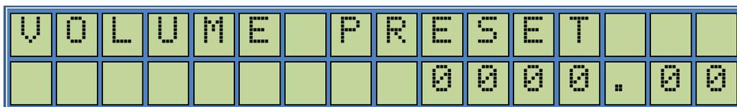
Likewise, using preset buttons the value pre-assigned will be added to the value on the screen and displayed both in the keyboard screen and volume field of the main display where, the sales part is automatically blanked out for better visibility.
