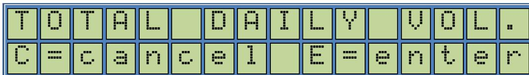
There are two reset able electronic totalizers in the calculator independent from the shift totalizers. These can be used by the manager, to reset after each desired period (ie Shift, Day, Week, Maintenance interval, etc.) First one is Daily Volume Totalizer.
