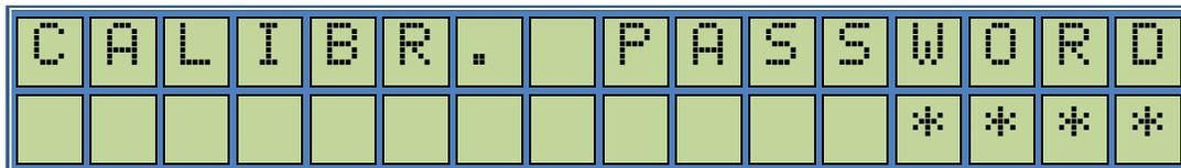
Enter your calibration password by using the number keys. The password is a 4-digit number and it should be followed by
