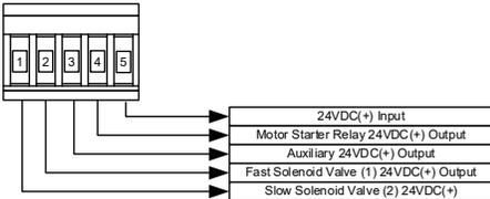
W&M Seal and Electromechanical Connector Bar (4 Pins) JP12, JP7
