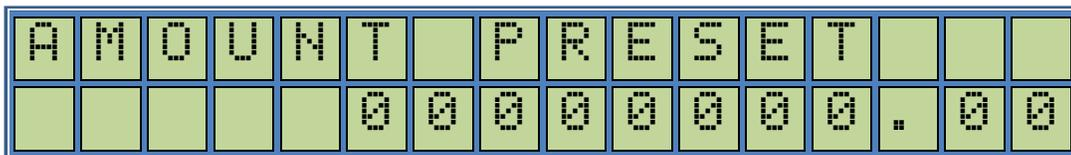
By using the number keys followed by the
