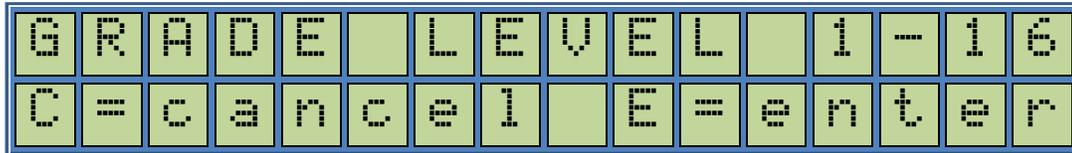
This is for setting the Grade Level. This is important if the dispenser is included into a communication chain. Default Grade Level is 01.
