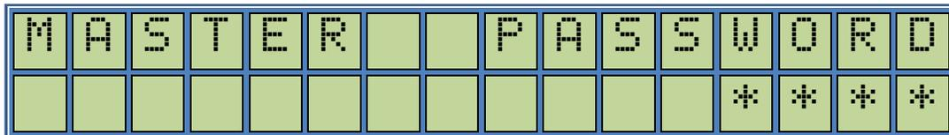
To enter into this menu, you need to type the 4 digit Master Password supplied with the dispenser. If you consult Service department for this password, you need to confirm the Version Number of the Software. Number keys will be used to enter the master password. If the password is wrong, an
